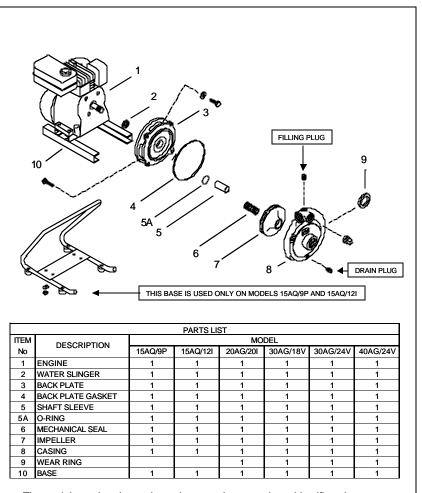
The serial number located on the pump's nameplate, identifies the pump's model and is required for reference when ordering spare parts.
