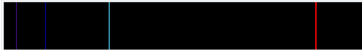
The four visible hydrogen emission spectrum lines in the Balmer series. H-alpha is the red line at the right.
