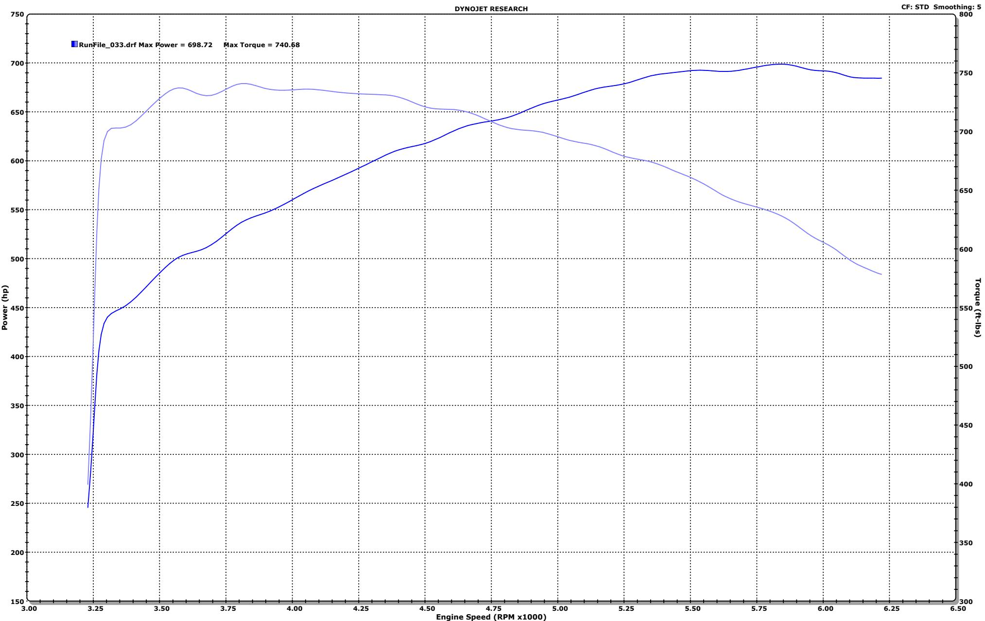
RunFile\_033.drf - 9/22/2016 3:32:01 PM Run Type: RO Run Conditions: 108.15 °F, 29.87 in-Hg, Humidity: 50%, STD: 1.07
